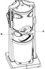
After exchanging their housings, reassemble the intake of the "A" suction pipe and the "B" closing plate by fastening the screws.
