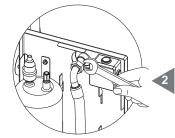
Screw the suction socket on the suction plug; check it has been firmly tightened.
