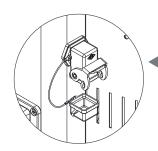
Disassemble the connector cover on the vacuum cleaner appliance.
