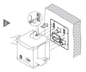
• 4.10 Disassembling the central nit from the installation template NOTE: This operation must be carried put ONLY in case of real need, e.g. for extraordinary repairing.
