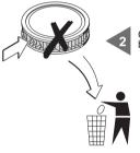
Check if the surface of the cartridge is torn; in this case, the filter cartridge cannot be used any longer.
