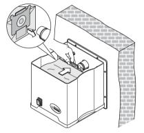
Place the new bag ATTENTION: gently move back and forward the bag so to fit the bag membrane into its slot
