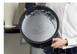
Powder container pre-separatorTurbix
