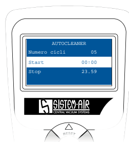
Autocleaner setting via Tecno Star Dual Power central vacuum cleaner display
