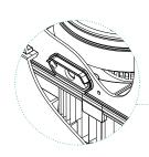
The **vacuum breaker valve** opens automatically, supplying air to the engine when the inlet flow from the intake pipe is reduced or absent, anticipating the intervention of the thermal protection.
